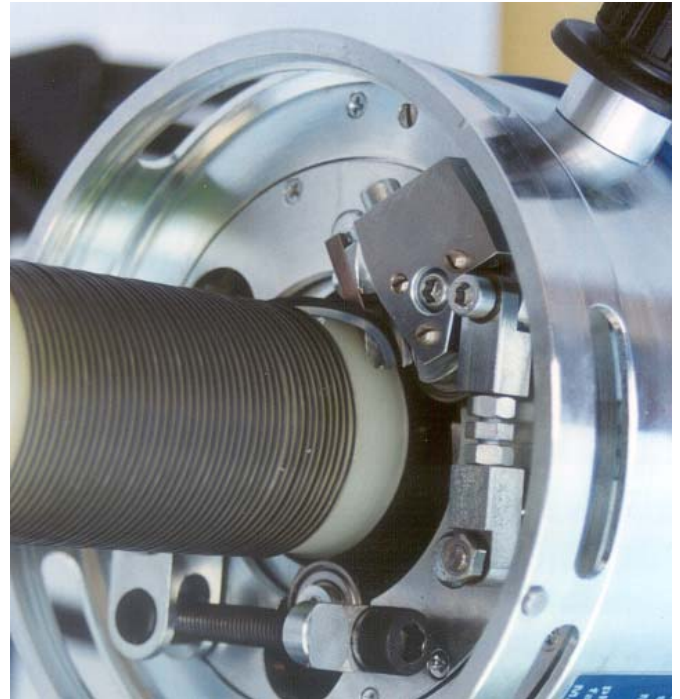
The motorized peeling tools of the Series S have become the standard solution for peeling long lengths to be inserted into water terminations.
